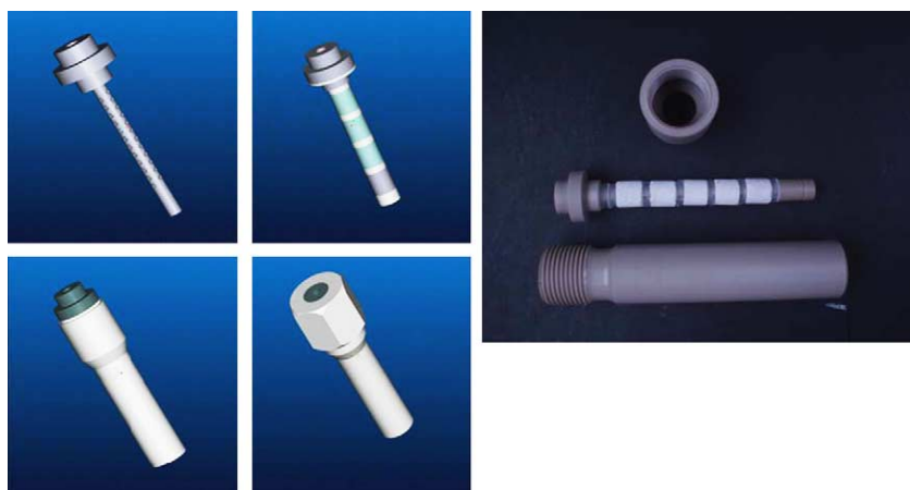
Fig. 3. Flow-through reactor with single ring shaped composites. Rings are aligned on a perforated tube. Gaskets between the rings prevent bypass. Housing is made of PEEK polymer. The flow streams from an annular gap through the ring walls and leaves through the perforated inner tube. Nine millimeters ring diameter.
