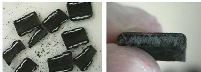
Fig. 5. Noble metal loaded rings by impregnation (only diffusion driven, left) and by convective forced flow through the ring wall (right).
