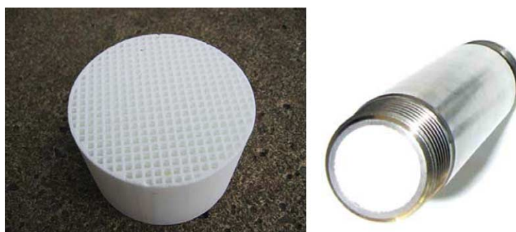
Fig. 2. Honeycomb monolithic composite (left), monolithic porous composite rod inserted into stainless steel tube (right). Diameter of the honeycomb monolith is 7.5 cm. Diameter of the stainless steel reactor is 2.4 cm, length of the inserted porous monolith is 11 cm.
