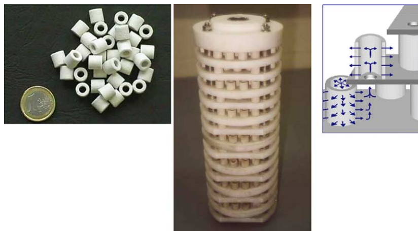
Fig. 1. Different polymer/carrier composites: Rings (upper left), rings in an arranged ordered structure (middle), flow pattern inside arranged rings (right), size of the arranged packing is about 20 cm in length.
